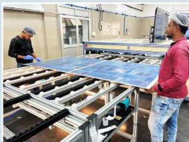
Layup & Bussing Station
